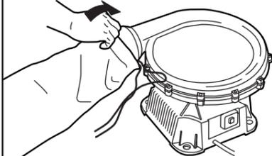
Attach longer fabric tube to blower unit making sure the tube is not twisted.
