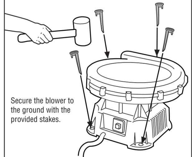
Secure the blower to the ground with the provided stakes.
